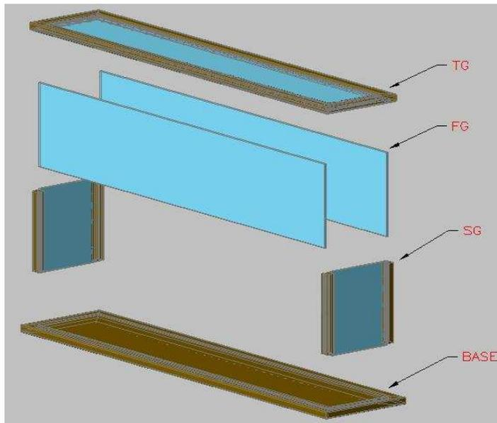
1. Unwrap each piece and remove the protection sheets from the acrylic sides. If your display has the mirror option, the grey side has no protective cover, only the reflective side does. Be sure that the reflective side is facing the inside of the case. If you ordered engraving to be done on the front panel, be sure the engraved side is also facing the inside of the display case.
